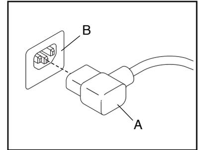
2. Plug the power cord into an appropriate outlet (C) that is properly installed and earthed in accordance with all local codes and ordinances.
